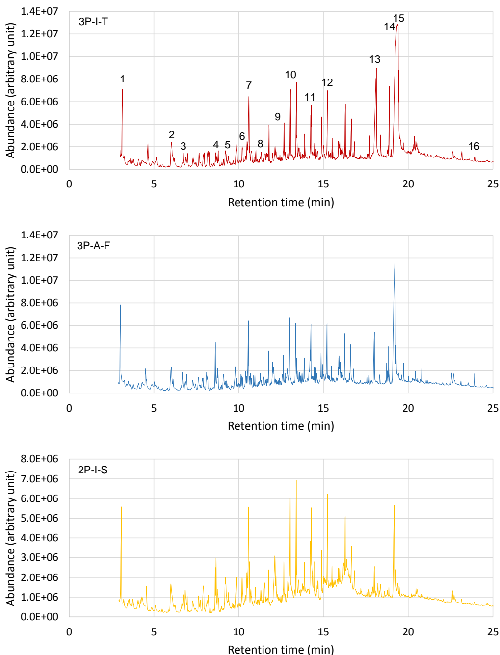
Figure 5: Py-GC/MS chromatograms of the three samples (3P-I-T, 3P-A-F, 2P-I-S).
