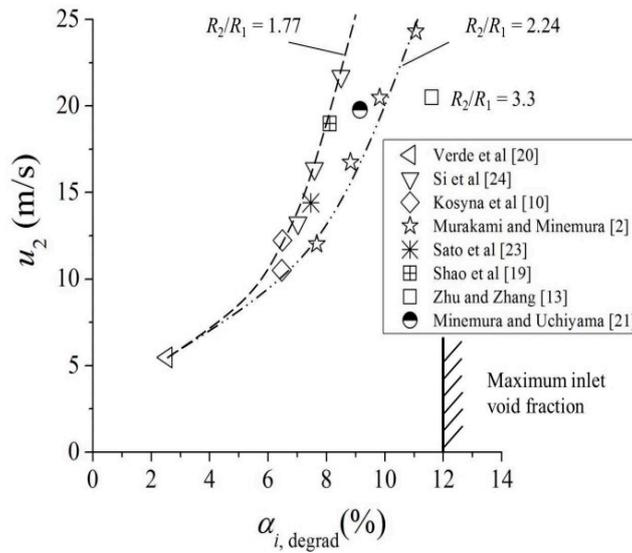
Figure 3. Effects of the impeller outlet rotational speed on the value of  $\alpha_{i,degrad}$ .
