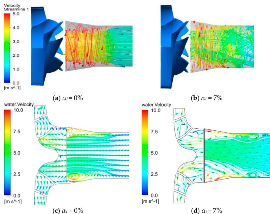
**Figure 5.** Local two-phase flow streamlines and meridional velocity vectors at impeller inlet and inside the impeller passage (not including impeller wall regions) at nominal rotational speed: 2910 rpm, and low flow coefficient  $\varphi = 0.038$  (nominal flow coefficient  $\varphi_n = 0.08$ ) for two different inlet void fractions: (a)  $\alpha_i = 0\%$ ; (b)  $\alpha_i = 7\%$ ; (c)  $\alpha_i = 0\%$ ; (d)  $\alpha_i = 7\%$ . Extracted from Si et al. [28].
