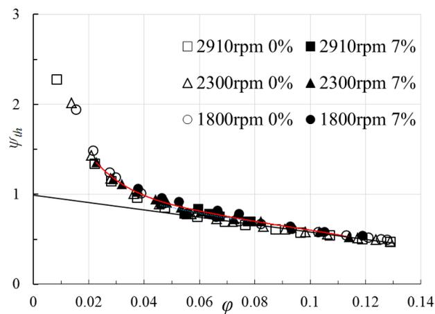
**Figure 10.** Theoretical head coefficient for different rotational speeds. (extracted from Si et al. [24]).
