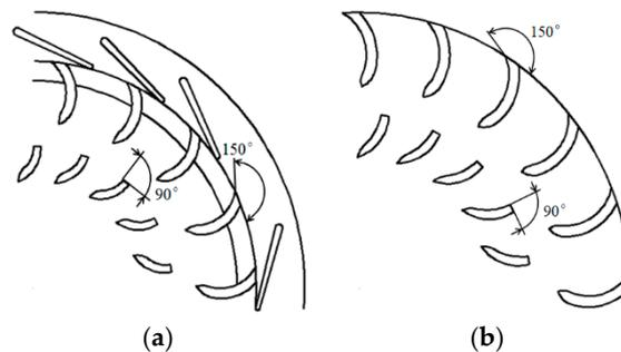
**Figure 12.** Example of particular pump designs using tandem blade arrangement (a) impeller diameter of 190mm with stator vanes; (b) impeller diameter of 235 mm without stator vanes (these figures have been reproduced from reference [34]).
