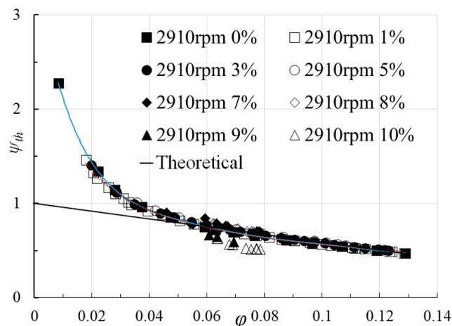
Figure 9. Theoretical head coefficient for nominal rotational speed (extracted from Si et al. [24]).
