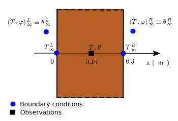
Figure 15: Illustration of the experimental design with the position of the sensors for the temperature, relative humidity and moisture content.
