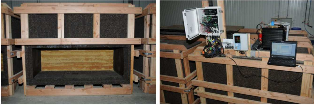
Figure 13: Overview of one of the boxes with an open door (on the left), and the central data-logger with the temperature and relative humidity control group (right) from [28].
