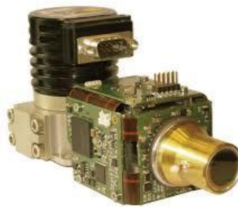
Figure 1 – T2SL MWIR IDDCA from IRnova.
