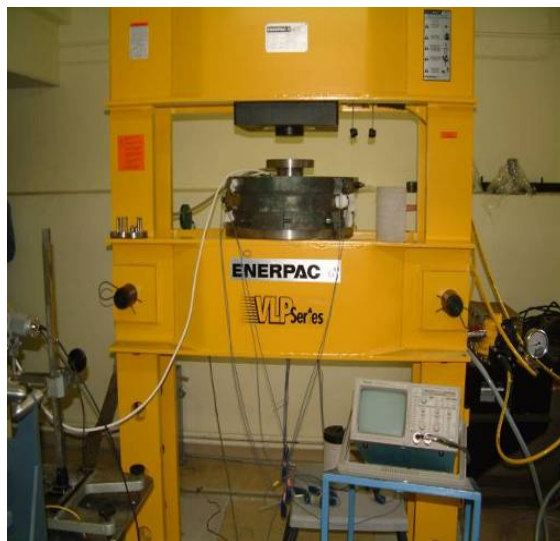
Figure 1.2. Hydraulic frame hosting the triaxial cell
