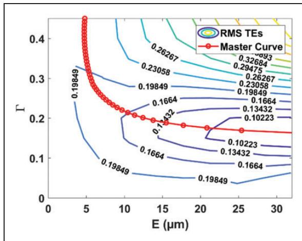
**Figure 18.** Effect of 10  $\mu\text{m}$  crowning on profile modification optimum (with centrifugal effects at  $\Omega_2 = 28,650 \text{ r/min}$  (3000 rad/s)).
