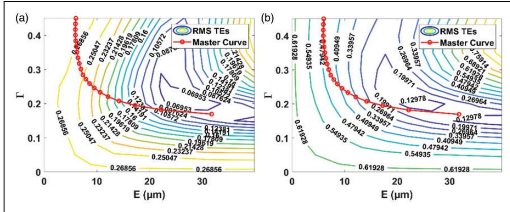
**Figure 12.** Effect of crowning on profile modification optimum (with centrifugal effects at  $\Omega_2$ ): (a)  $A = 10 \mu\text{m}$ ; (b)  $A = 20 \mu\text{m}$ . RMS TEs: root mean square transmission errors.
