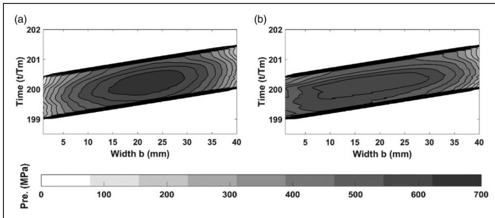
**Figure 16.** 10 µm crowning for both studied speed with both flexible pinion and wheel. (a)  $\Omega_1$  and (b)  $\Omega_2$ .
