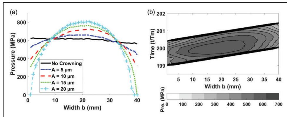
**Figure 8.** Crowning effect on pressure distribution at middle-range speed (14,325 r/min (1500 rad/s)): (b)  $A = 5 \mu\text{m}$ .
