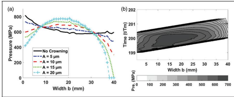
**Figure 9.** Crowning effect on pressure distribution at high speed (28,650 r/min (3000 rad/s)): (b)  $A = 10 \mu\text{m}$ .
