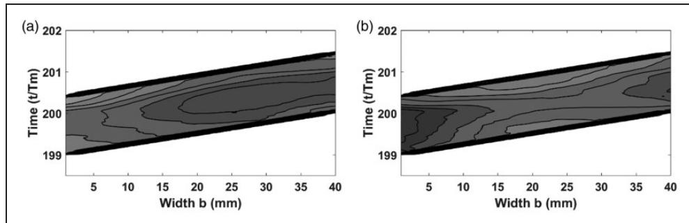
**Figure 14.** Centrifugal effect influence on pressure distribution for fully webbed gear: (a)  $\Omega_2$ , without centrifugal effects; (b)  $\Omega_2$ , with centrifugal effects.
