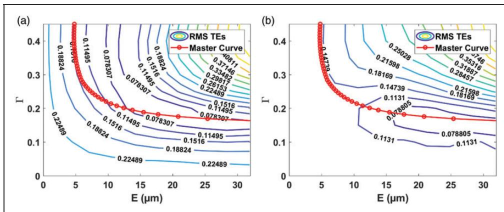
**Figure 17.** Optimisation with regard to the TEs for: (a) centrifugal effects at zero speed and (b) centrifugal load for  $\Omega_2 = 28,650$  r/min (3000 rad/s).
