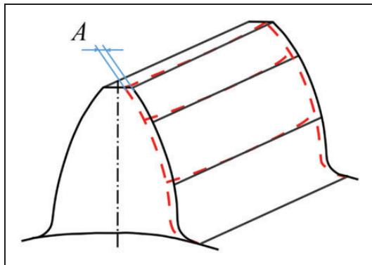
**Figure 7.** Crown definition ( $A$  is the crown amplitude).
