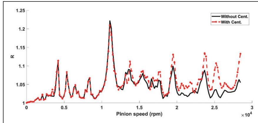
**Figure 4.** Dynamic tooth load factor with and without centrifugal effects (thin-rimmed gear).
