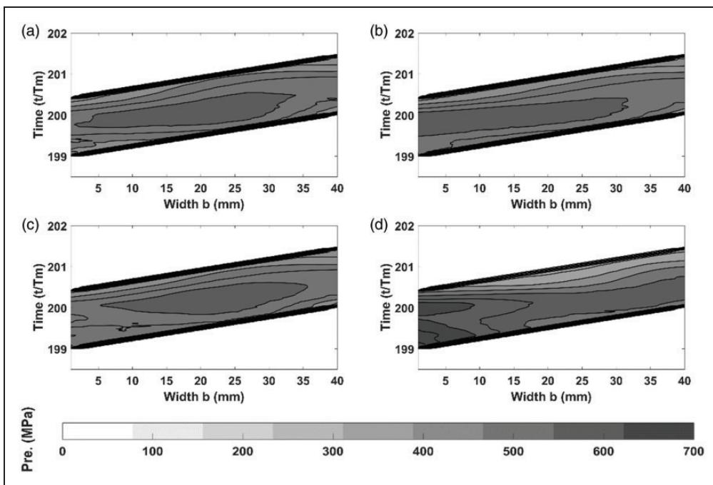
**Figure 5.** Centrifugal effect influence on pressure distribution: (a)  $\Omega_1$ , without centrifugal effects; (b)  $\Omega_1$ , with centrifugal effects; (c)  $\Omega_2$ , without centrifugal effects; (d)  $\Omega_2$ , with centrifugal effects.
