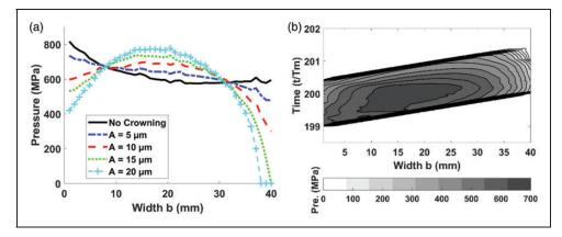
Figure 9. Crowning effect on pressure distribution at high speed (28,650 r/min (3000 rad/s)): (b)  $A = 10 \,\mu$ m.
