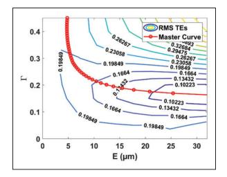
Figure 18. Effect of 10  $\mu$ m crowning on profile modification optimum (with centrifugal effects at  $\Omega_2 = 28,650$  r/min (3000 rad/s)).
