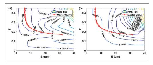
**Figure 11.** Optimisation with regard to the TEs for: (a) centrifugal effects at zero speed and (b) centrifugal load for  $\Omega_2 = 28,650 \text{ r/min (3000 rad/s)}.$
