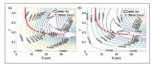
**Figure 12.** Effect of crowning on profile modification optimum (with centrifugal effects at  $\Omega_2$ ): (a)  $A = 10 \,\mu\text{m}$ ; (b)  $A = 20 \,\mu\text{m}$ . RMS TEs: root mean square transmission errors.
