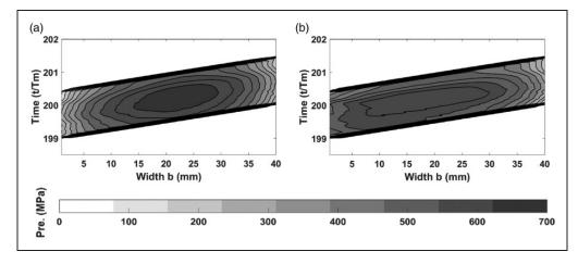
Figure 16. 10  $\mu$ m crowning for both studied speed with both flexible pinion and wheel. (a)  $\Omega_1$  and (b)  $\Omega_2$ .
