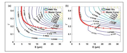
**Figure 17.** Optimisation with regard to the TEs for: (a) centrifugal effects at zero speed and (b) centrifugal load for  $\Omega_2 = 28,650 \text{ r/min}$  (3000 rad/s).
