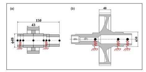
**Figure 2.** (a) Pinion geometry with beam model; (b) thin-webbed gear definition, modelled with condensed FE – springs represent casing/bearings, torsional springs represent splines (resisting torque).
