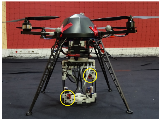
Fig. 2: The quadrotor UAV used for the SP Cup, equipped with a 3D-printed 8-microphone array. Circles highlight two of the microphones.
