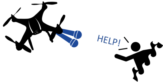
Fig. 1: Microphones embedded in a UAV may help localizing people for search and rescue in disaster areas.
