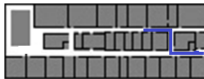
Figure 2 Altran indoor map, the blue line corresponds to the closest path using the Dijkstra algorithm.
