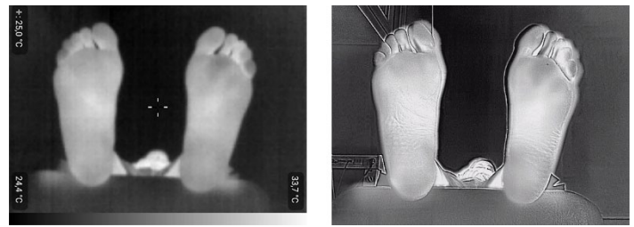
Figure 3: Example of plantar feet surface image taken with a Flir One Pro camera. Thermal mode (a), MSX mode (b).
