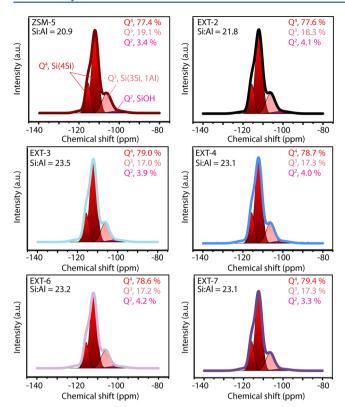
**Figure 4.** Direct-excitation <sup>29</sup>Si solid-state MAS NMR spectra of parent zeolite ZSM-5 and shaped zeolite ZSM-5 extrudates prepared with varying formulations. Si-species identified as  $Q^4$  (-112 and -116 ppm),  $Q^3$  (-106 ppm), and  $Q^2$  (-100 ppm), with corresponding Si:Al calculated (cf., eq 1).
