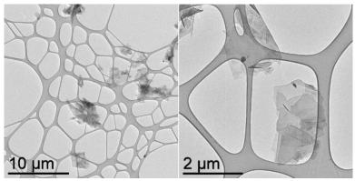
Figure 1. Transmission Electronic Microscopy of dried FLG.
