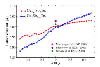
FIG. 3. Lattice parameter calculated with VASP for the GST compounds  $Ge_{2+x}Sb_2Te_5$  (in red) and  $Ge_2Sb_{2+y}Te_5$  (in blue). Three experimental results are also indicated for  $Ge_2Sb_2Te_5$ .
