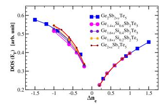
FIG. 13. Density of electron states at  $E_F$  as a function of  $\triangle n_e$  for  $Ge_{2+x-z}Sb_2Si_zTe_5$  crystals with z=0.0 (red), 0.2 (orange), 0.4 (violet), and 0.6 (magenta), and for  $Ge_2Sb_{2+y}Si_zTe_5$  crystals (blue).
