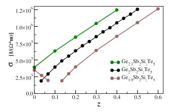
FIG. 10. Electrical conductivity of  $\mathrm{Ge_{2+x}Sb_2Si_zTe_5}$  compounds calculated for x=-0.1 (in brown), x=0.0 (in black), and x=0.1 (in green) versus concentration of dopant Si atoms.
