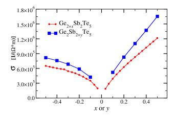
FIG. 7. Electrical conductivity of  $Ge_{2+x}Sb_2Te_5$  (in red) and  $Ge_2Sb_{2+y}Te_5$  (in blue) GST compounds, as a function of the Ge or Sb concentration.
