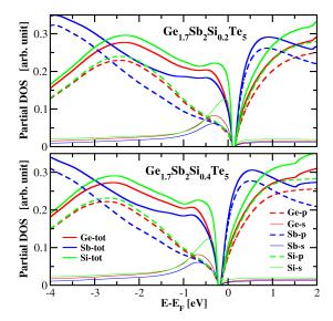
FIG. 9. Contribution of single Ge, Sb, and Si atoms to the DOS of  $Ge_{1.7}Sb_2Te_5$  crystals doped with different concentrations of Si atoms. The s and p partial DOS curves are also shown. Upper and lower panels respectively correspond to  $Ge_{1.7}Sb_2Si_{0.2}Te_5$  and  $Ge_{1.7}Sb_2Si_{0.4}Te_5$ .
