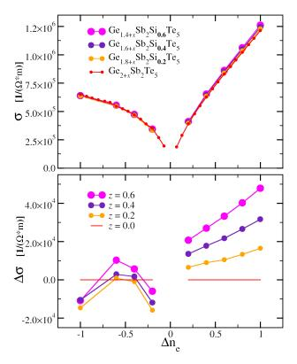
FIG. 12. Top: electrical conductivity of  $\mathrm{Ge}_{2+x-z}\mathrm{Sb}_2\mathrm{Si}_z\mathrm{Te}_5$  crystals for z=0.0 (red), 0.2 (orange), 0.4 (violet), and 0.6 (magenta), as a function of  $\Delta\mathrm{n}_e$ . Bottom: for the same systems, difference between these conductivities and the conductivity of  $\mathrm{Ge}_{2+x}\mathrm{Sb}_2\mathrm{Te}_5$ .
