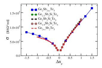
FIG. 11. Conductivity of  $Ge_{2+x}Sb_{2+y}Si_zTe_5$  crystals as a function of  $\triangle n_e$ , the difference in their number of p-valence electrons per formula unit with respect to  $Ge_2Sb_2Te_5$ .
