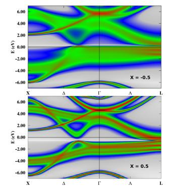
FIG. 5. Bloch Spectral Function calculated with the code SPRKKR for the GST compounds  $Ge_{2+x}Sb_2Te_5$  with x = -0.5 (upper panel) and x = 0.5 (lower panel). E=0 corresponds to the Fermi level. The color coding is the same as in fig. 4.
