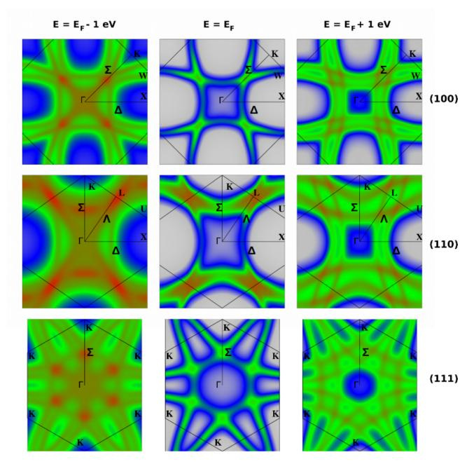
FIG. 6. Map of the Bloch Spectral Function calculated with the code SPRKKR for three different planes of the first BZ of  $Ge_{2.005}Sb_2Te_5$ : (100) in upper-row panels, (110) in middle-row panels, and (111) in lower-row panels, and for each of them at three different energies:  $(E_F - 1 \text{ eV})$  on the left side,  $E_F$  in the middle, and  $(E_F + 1 \text{ eV})$  on the right side. The color coding is the same as in fig. 4.
