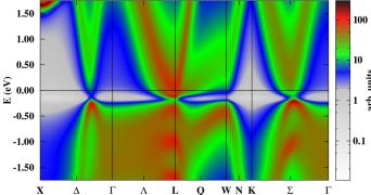
FIG. 4. Bloch Spectral Function calculated for Ge<sub>2.005</sub>Sb<sub>2</sub>Te<sub>5</sub> with the code SPRKKR, shown on a wide energy range (left side), and for energies near the Fermi level (right side). E=0 corresponds to the Fermi level.
