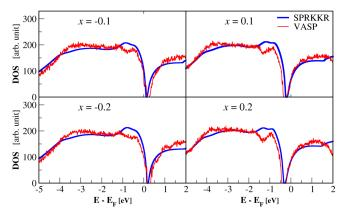
FIG. 2. Left: Density of states calculated with the codes SPRKKR (blue lines), and VASP (red lines) for GST compounds  $Ge_{2+x}Sb_2Te_5$  with x = -0.2, -0.1, 0.1,and 0.2. Right: Same results, but for energies near the fermi level.
