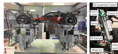
Fig. 4. The experimental testbed INOVE at GIPSA-lab (see www.gipsa-lab.fr/projet/inove )
