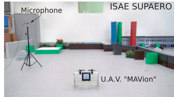
Figure 19. Indoor flying platform at ISAE-SUPAERO and flight test of MAV with optimized rotor.
