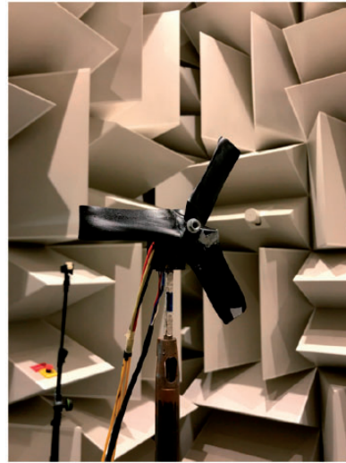
Figure 13. Experimental set-up in the anechoic chamber used to validate the ISO standard. The five components aerodynamic balance is below the motor driving the rotor.
