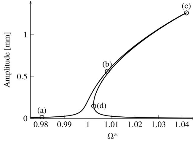
Fig. 3: FREQUENCY RESPONSE AT BLADE TIP NEAR  $\omega_1$
