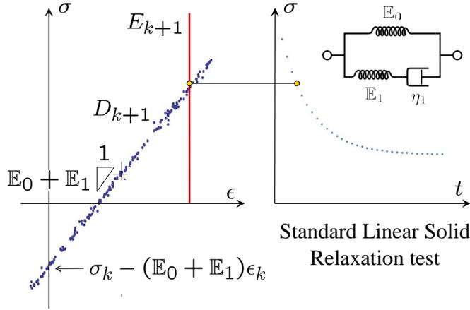
FIGURE 1. Schematic representation of the relaxation test for a Standard Linear Solid bar. Inlaid expressions shown in the limit  $\Delta t \rightarrow 0$  for simplicity. The constraint set  $E_{k+1}$ , left, is fixed at a constant strain while the data set  $D_{k+1}$  moves downward parallel to itself so as to trace the relaxation curve of the bar, right.
