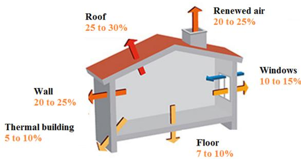
Figure 2. Medium energy loss for houses built before 1974
