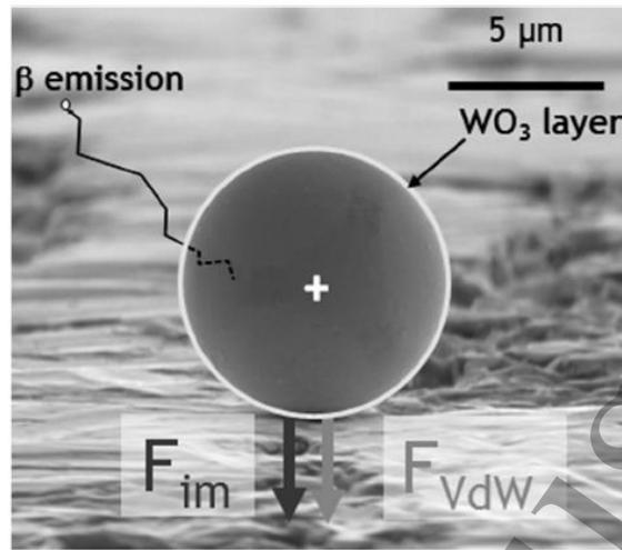
FIG. 6. Schematic of balance of forces in the case of a W spherical tritiated particle lying on a W surface
