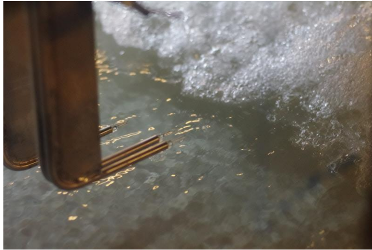
Figure 2. High-speed photograph (shutter speed: 1/2,000 s) of probe array immediately before roller impact, with bore direction from top right to bottom left, during the physical experiments—The reference probe is on the far left
