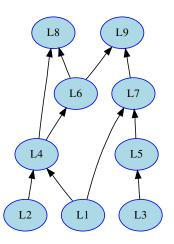
Figure 1: The result of the -vec option is a directed acyclic graph (DAG) of small computation loops
