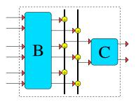
Figure 4: sequential composition when  $\mathbf{outs}(B) = k *$ ins(C)
