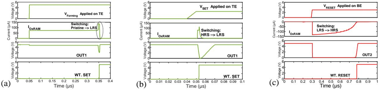
Fig. 4. Simulations waveforms of: applied voltage ( $V_{\text{Forming}}$ ,  $V_{\text{SET}}$  and  $V_{\text{RESET}}$ ), current through OxRAM ( $I_{\text{OxRAM}}$ ), voltage on OUT1 and OUT2 nodes, WT.SET and WT.RESET signals during (a) Forming, (b) SET and (c) RESET operations.
