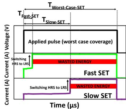
Fig. 2. Current and voltage waveforms during SET operation with different switching times ( $T_{\text{Fast-SET}}$  and  $T_{\text{Slow-SET}}$ ). Programming pulse width covers the worst-case SET time ( $T_{\text{Worst-Case-SET}}$ )
