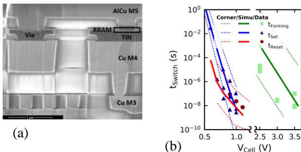
Fig. 1. (a) TEM cross section of TiN/HfO<sub>2</sub>/Ti/TiN OxRAM [21]. (b) Measured switching times  $t_{\text{Forming}}$ ,  $t_{\text{Set}}$  and  $t_{\text{Reset}}$  versus applied programming voltage  $V_{\text{Cell}}$  (symbols), and the corresponding simulation results with corners (lines). Experimental data were measured on the adopted OxRAM technology in [9,22].
