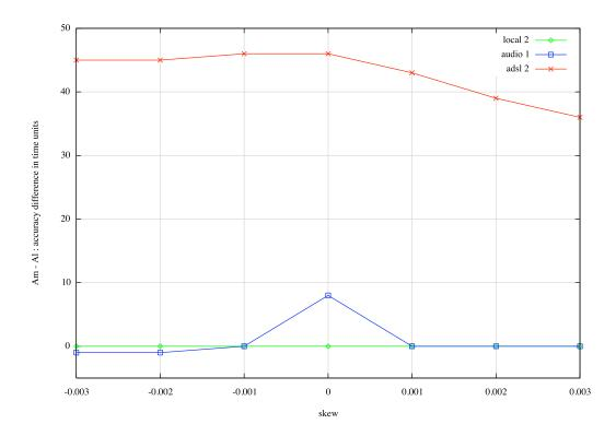
Figure 4: Mid point versus low point comparison: the graphic shows the accuracy difference between the mid and low point averaging.
