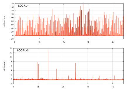
Figure 11: Ping measurements over a local Ethernet network. The first transmission has been measured on a general purpose 10Mb Ethernet network. The second transmission has been measured on Ethernet 100Mb isolated by a switch.
