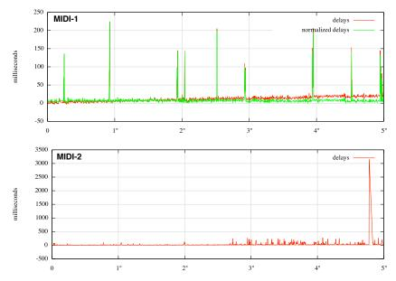
Figure 13: MIDI transmission over Internet via a modem line. For the second transmission, note the latency change starting at 3". Note also that the normalized delays are not plotted because they were not significant.
