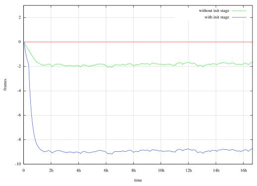
Figure 5: ADSL1 skew estimation with and without initial stage.
