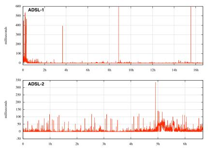
Figure 10: Ping measurements over Internet via adsl. The first transmission exhibits a high delay period at the session start time. The second transmission shows a significant delay increase starting at hour 5.
