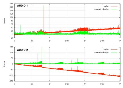
Figure 12: Audio buffers transmission over Ethernet. 4 different stations were involved. Measurements of 2 stations are presented along with the corresponding normalized delays.
