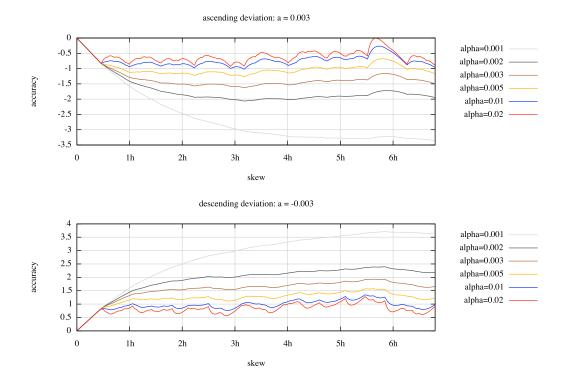
Figure 7: Normalized skew estimations with varying  $\alpha$  factor.
