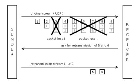
Figure 3: Redundancy and retransmission
