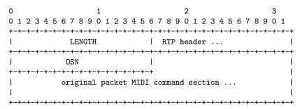
Figure 7: Retransmission packet structure
