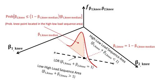
Figure 4. Schematic representation of the probabilistic position of the knee-point and the loading
