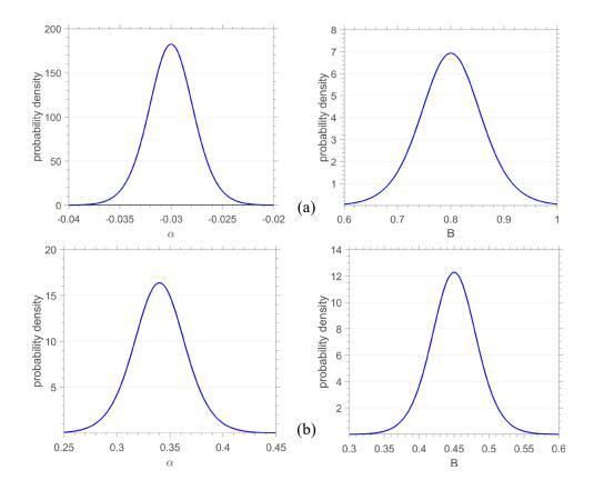
**Figure 10.** Estimated MaxEnt distributions of the DLDR input variables α and *B* using the two-load experimental dataset obtained from: (a) Tanaka, and (b) Xie045.
