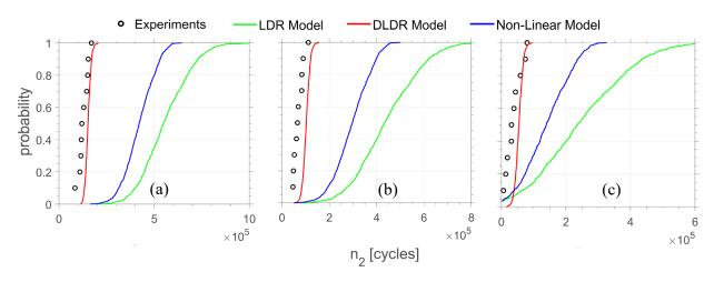
Figure 14. Experimental remaining fatigue life from Xie16Mn H-L experiments and probability distributions predicted with DLDR, LDR and non-linear models: (a)  $n_1$ =26,000 cycles; (c)  $n_1$ =44,000 cycles, and (d)  $n_1$ =75,000 cycles.
