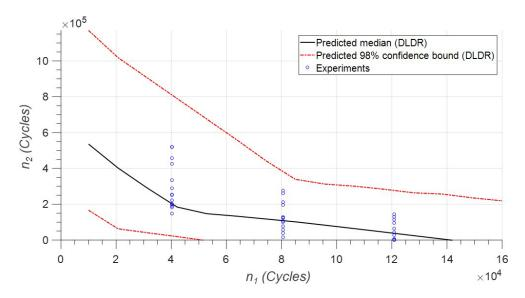
Figure 16. Probabilistic  $n_2$  vs.  $n_1$  using DLDR for the Xie045 data.
