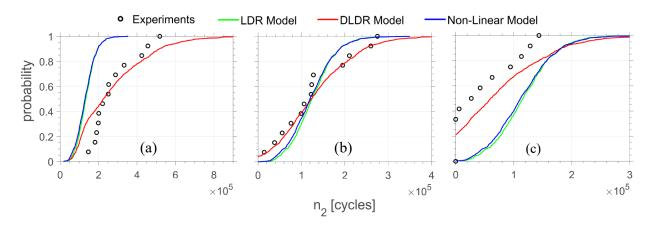
Figure 13. Experimental remaining fatigue life from Xie045 H-L experiments and probability distributions predicted with DLDR, LDR and non-linear models: (a)  $n_1$ =40,300 cycles; (b)  $n_1$ =80,600 cycles, and (c)  $n_1$ =120,900 cycles.
