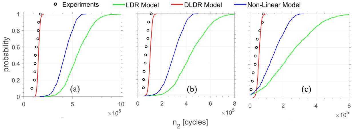
**Figure 14.** Experimental remaining fatigue life from Xie16Mn H-L experiments and probability distributions predicted with DLDR, LDR and non-linear models: (a)  $n_1=26,000$  cycles; (c)  $n_1=44,000$  cycles, and (d)  $n_1=75,000$  cycles.
