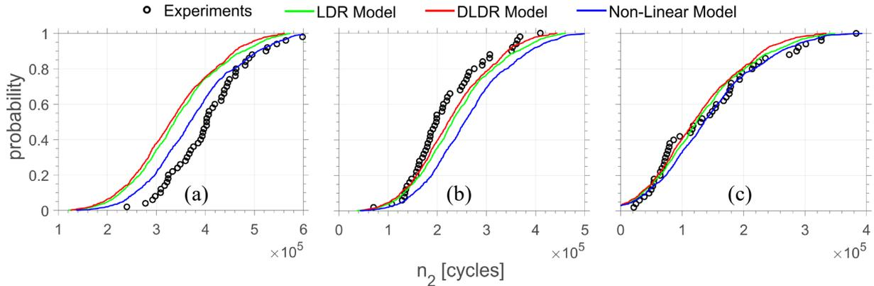
**Figure 12.** Experimental remaining fatigue life from Tanaka H-L experiments and the probability distributions predicted with the DLDR, LDR, and non-linear models: (a)  $n_1=13,300$  cycles; (c)  $n_1=26,500$  cycles, and (d)  $n_1=39,800$ .
