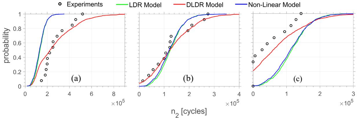
**Figure 13.** Experimental remaining fatigue life from Xie045 H-L experiments and probability distributions predicted with DLDR, LDR and non-linear models: (a)  $n_1=40,300$  cycles; (b)  $n_1=80,600$  cycles, and (c)  $n_1=120,900$  cycles.
