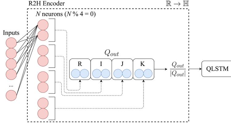
Figure 1: Illustration of the R2H encoder, used as an input layer to a QLSTM. Inputs are real, before being turned into quaternions, and finally unitary quaternions within the R2H encoder.
