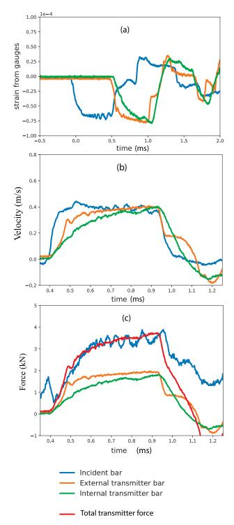
Figure 3: Measurements from bars: (a) strain from gauges, (b) velocities, and (c) forces in bars
