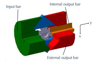
Figure 1: Set-up principle for dynamic equibiaxial compression test.
