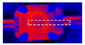
(b) Observation zone for a 15000 Hz infrared recording  $(64 px \times 8 px)$
