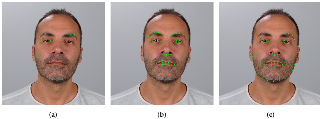
Figure 4. Face landmark detection: an example of output of three face landmark detectors. Face image extracted from the IST-EURECOM Light-Field Face Database (LFFD). (a) CLandmarks [40]; (b) IntraFace [41]; (c) DLIB.
