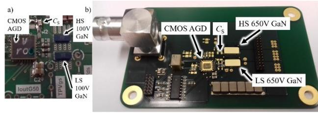
Fig. 4. AGD in a half bridge configuration for test in double pulse for (a) 4-layer board with 48V DC bus voltage with 100V GaN EPC 2001C device. (b) 6-layer board with 400V DC bus voltage with 650V GaN systems GS66508T devices.
