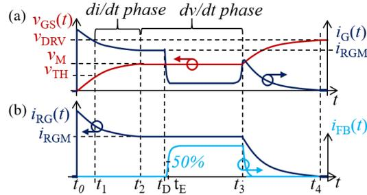
Fig. 2. Qualitative waveforms for gate voltage and currents with the AGD during turn-on (closed-loop). (a) Current and voltage at the power gate and (b) currents being supplied and sinked simultaneously by the AGD.
