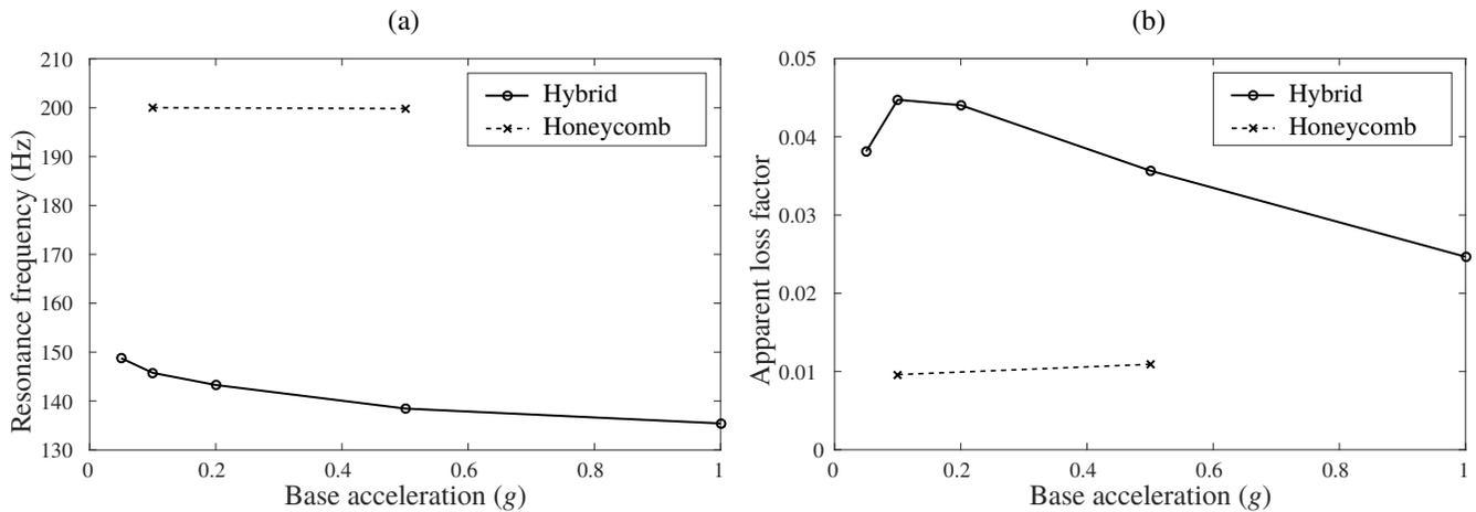
**Figure 18.** Evolution of (a) the resonance frequency and (b) the apparent loss factor with respect to the base acceleration level for the first bending mode of the hybrid beam and the honeycomb beam B
