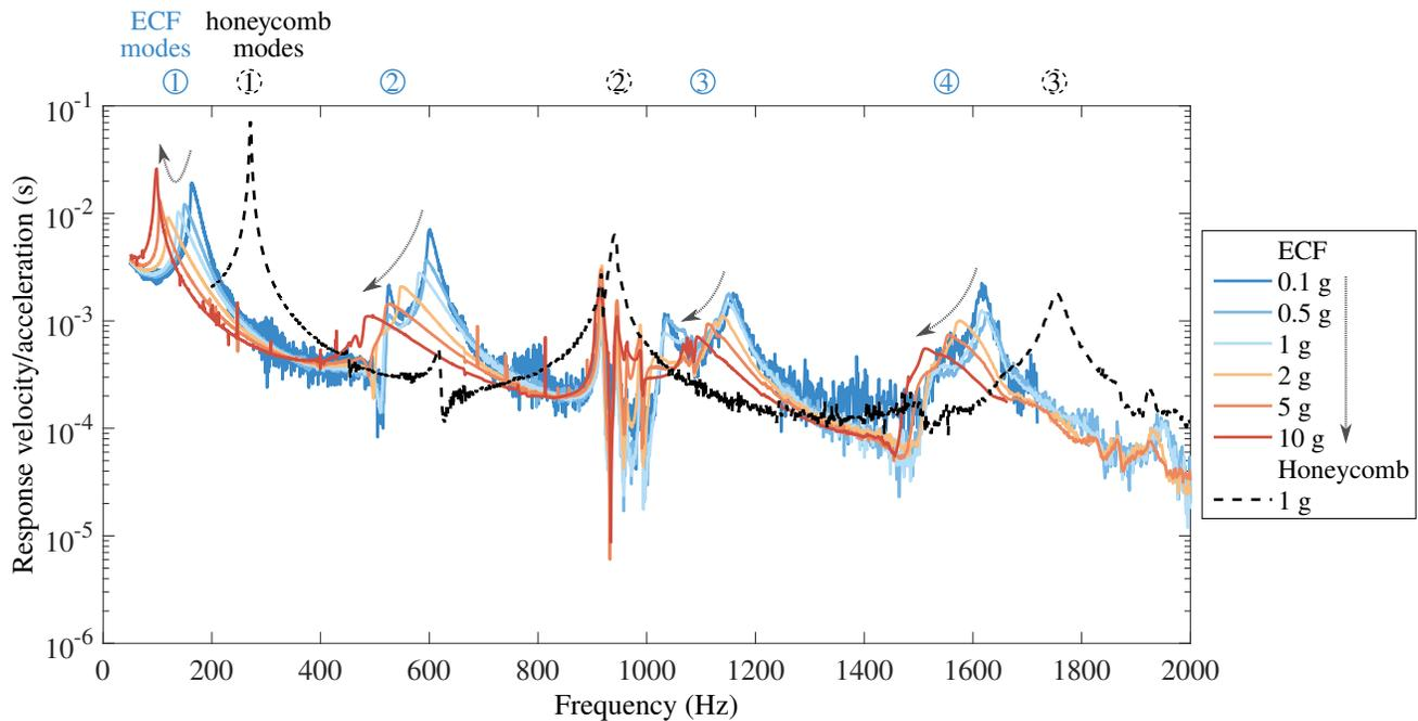
**Figure 14.** Frequency response of the ECF beam and the honeycomb beam A on a larger frequency range, with corresponding mode numbers in circles
