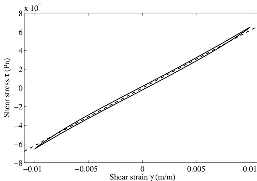
**Figure 2.** Measured hysteresis loop for shear strain amplitude  $\gamma_0 = 1 \cdot 10^{-2}$  at frequency  $f = 20$  Hz [10]; the dashed line corresponds to  $\tau = G_1\gamma$  with  $G_1 = 6.2 \cdot 10^6$  Pa
