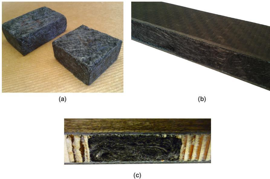
**Figure 21.** Consequences of the fabrication process on the sample sides: (a) small samples with adapted moulds, (b) full ECF core beam with adapted mould and (c) ECF insert in the hybrid beam cut from a larger sample.
