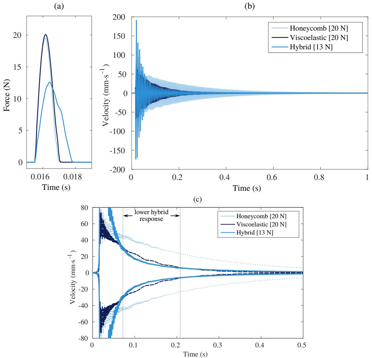
**Figure 20.** Response to an impact: (a) impact force signal for all beams, with the same impulse level, (b) time response of the beams and (c) envelopes of the responses, zoom on lower amplitudes of vibration
