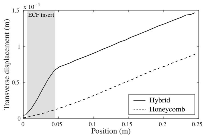
**Figure 19.** Transverse displacement of the hybrid beam and honeycomb beam B under a 0.5 g base acceleration; the change in slope for the hybrid beam occurs at the junction between the ECF insert (in grey) and the honeycomb core
