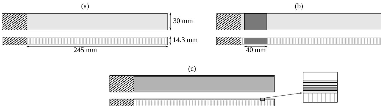
Figure 7. Three beams tested to assess the effect of a hybrid honeycomb/fibrous core on sandwich beam damping, top and side views: (a) reference honeycomb beam B, no damping treatment, (b) beam with hybrid honeycomb/fibrous core, and (c) beam with viscoelastic inserts
