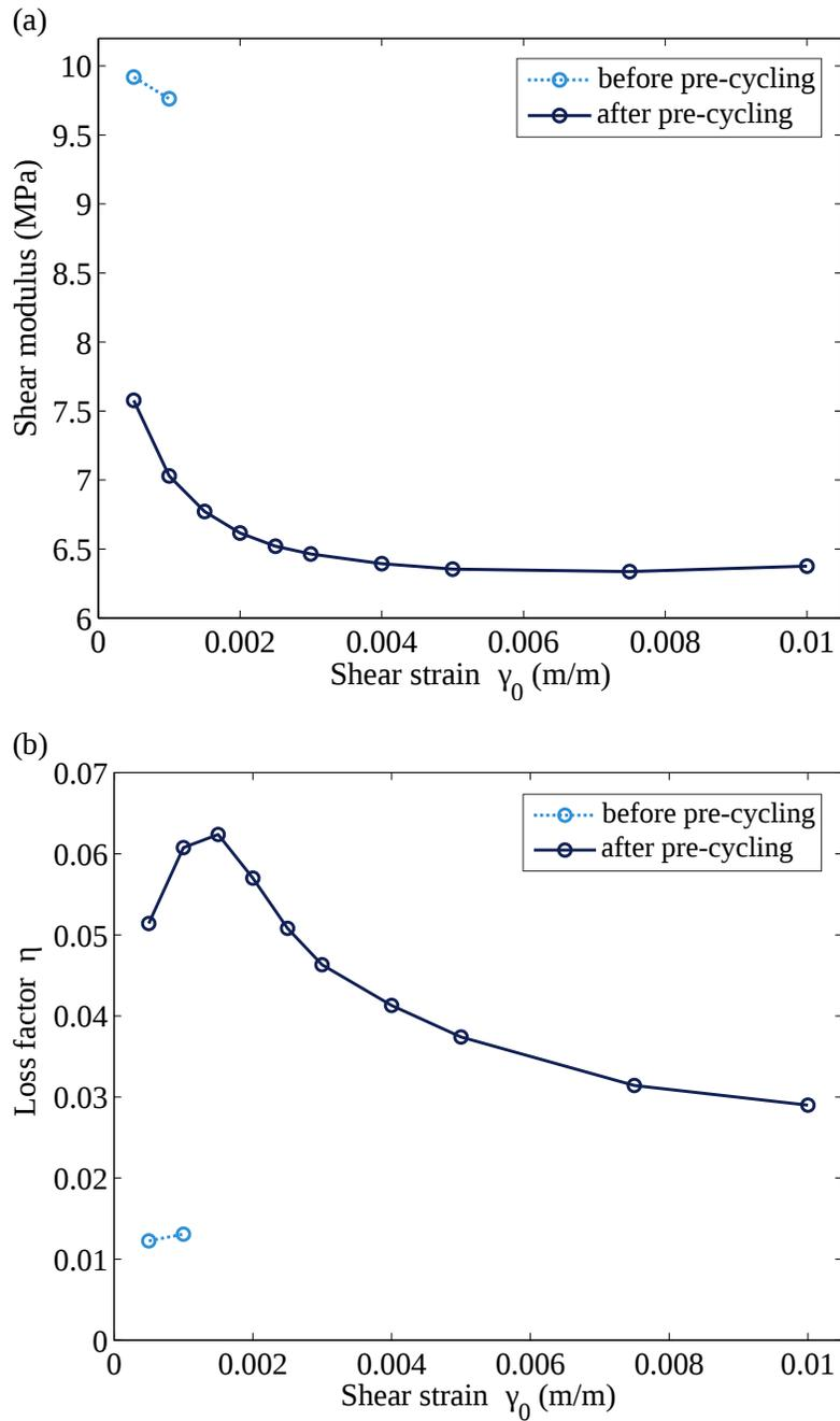
Figure 4. Evolution of (a) shear modulus and (b) loss factor with pre-cycling, with respect to shear strain amplitude
