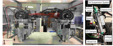
Fig. 5. The experimental testbed INOVE at GIPSA-lab (see www.gipsa-lab.fr/projet/inove )
