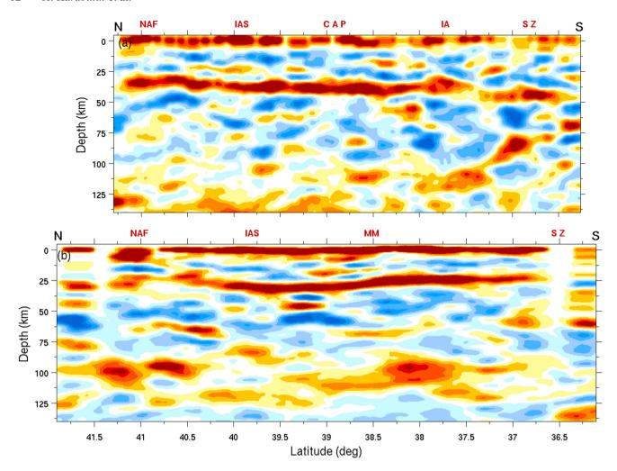
Figure 3. Migrated depth sections of radial receiver function records along two north—south profiles in Western Anatolia. (a) Eastern profile at longitude 30.5°E (b) Western profile at longitude 28°E. No vertical exaggeration. CAP, Central Anatolian Plateau; IA, Isparta Angle; SZ, Subduction Zone; IAS, Izmir-Ankara Suture; MM, Menderes Massif; NAF, North-Anatolian Fault.
