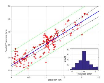
**Figure 4.** Crustal thickness versus topography sampled at station locations shown in Fig. 2(a) between  $37^{\circ}N-41^{\circ}N$  and  $27^{\circ}E-42^{\circ}E$ . The thick blue line is h = (T-26)/9.4.  $R^2$  is estimated as 0.82. The thin dashed black lines indicate 95 per cent confidence intervals of the blue line while the green dashed lines indicate 95 per cent prediction intervals. Inset figure shows the distribution of crustal thickness deviations from the regression.
