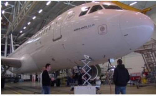
Fig. 9. Deployment of the positioning system after an human operator request in order to scan an A320 aircraft at Air France Industries.
