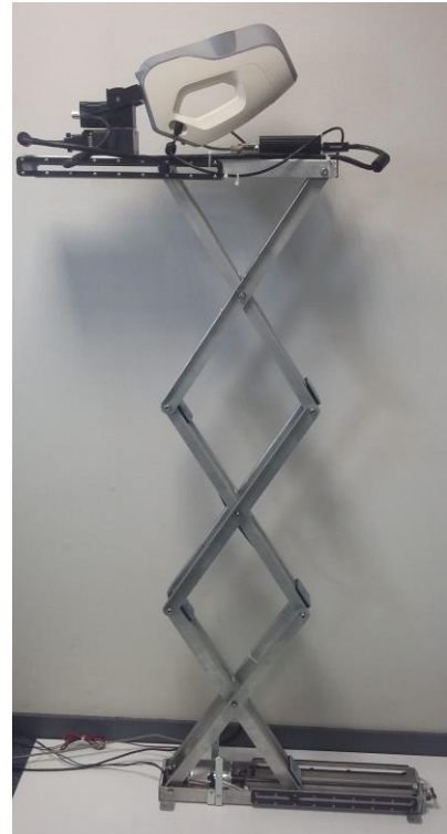
Fig. 11. Unfolded scanner positioning system.
