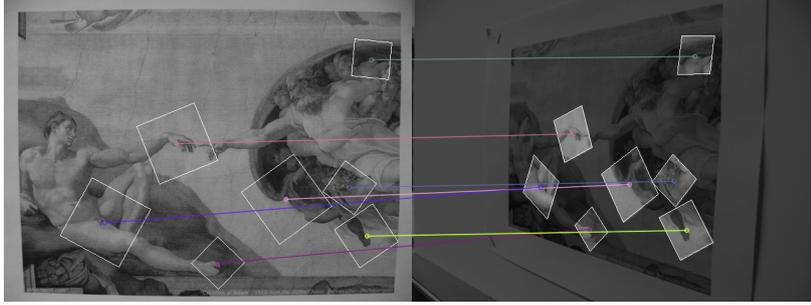
Figure 1: Some correspondences together with local affine maps estimated by the proposed LATE network. Patches on the target are warped versions of their corresponding query patch.
