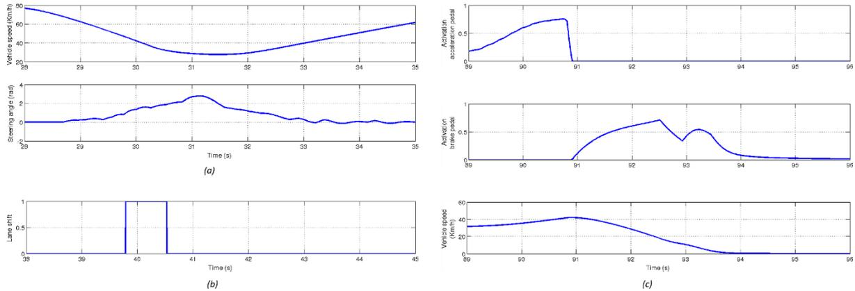
**Figure 8** Time series of monitored variables from experiments of Figure 7. (a) Smooth speed decrease and action on the steering angle of vehicle of Figure 7(a). (b) Lane shift of vehicle of Figure 7(b). (c) Actions on acceleration and brake pedals of vehicle of Figure 7(c), and consequent smooth decrease of vehicle speed.
