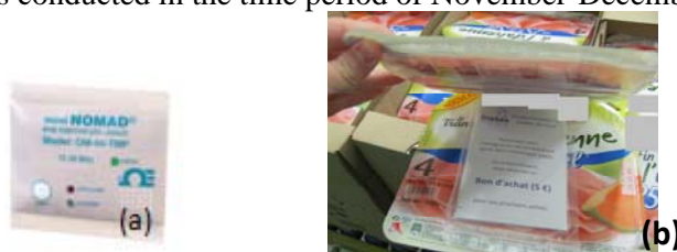
Picture 2. (a) Data logger inserted in the food package in order to record time-temperature data of the cold chain and (b) MAP cooked ham slices package used in the field test conducted in France.
