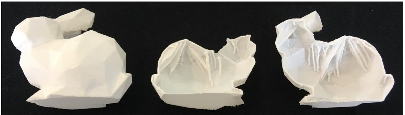
**Figure 1:** Hollowed Bunny printed with our method, using only 2.2% of material inside (compared to a filled model). **Left:** The full model. **Middle and right:** Same model cut in half, revealing the internal support structures generated by our approach (the supports use 316mm of filament over a total of 1622mm for the print). Bunny model (size: 54 × 43 × 53 mm). Support generation took 34 seconds. Printing time 1h 5min 30sec.
