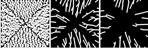
Figure 9: Three slices ( BS_i ) for a hollowed cube (from higher to lower). The initial support trees quickly merge into the outer walls.
