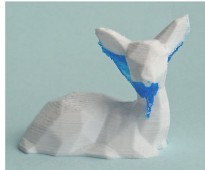
Figure 27: Half-size fawn model, printed with our method for external support, using a blue filament color for supports.
