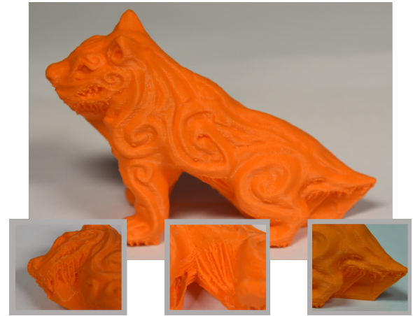
Figure 26: Demon dog printed using our method for external support.
