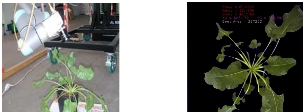
Figure 10 - Detection of sugar beet leaves by image processing
