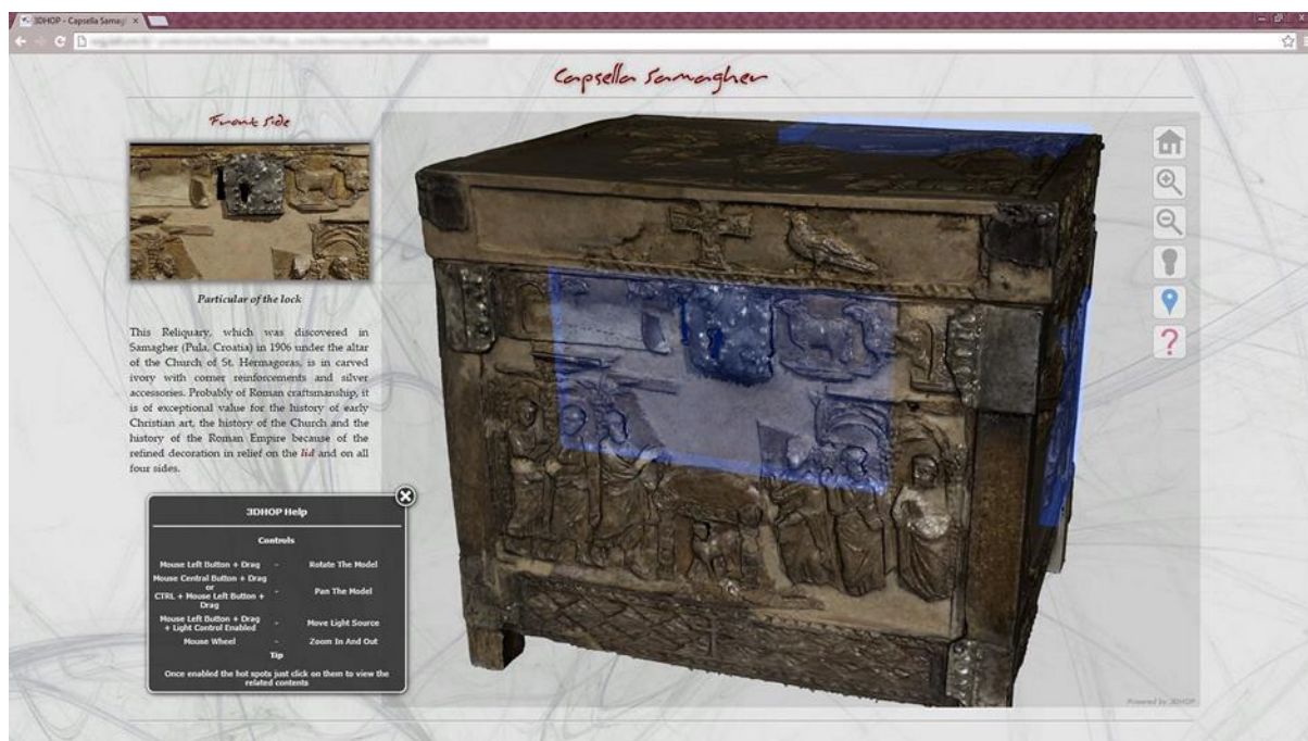
Figure 4: A 3DHOP application developed by CNR-ISTI. In this example, a high-resolution 3D digitization (10 million triangles) of the Capsella Samagher, an antique reliquary, is presented with additional information (images and text). These information are linked to the 3D geometry through geometric hotspots (light-blue regions).
