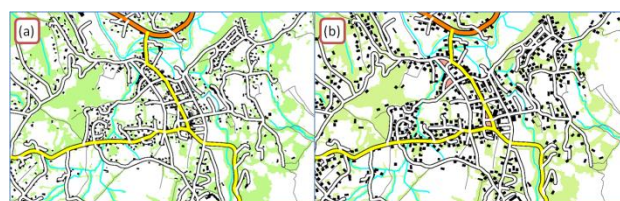
Figure 13. A small town at 1:50k before and after generalization, reducing blank space in the map
