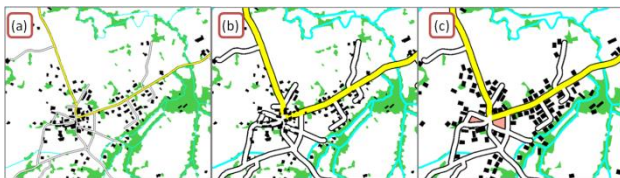
Figure 4. (a) initial data at 1:15k with a symbols scaled to 1:15k. (b) same data with symbols scaled to 1:25k. (c) data generalized to 1:25k
