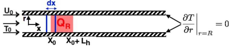
Figure 9: Simplified domain: Cylindrical duct with adiabatic walls.
