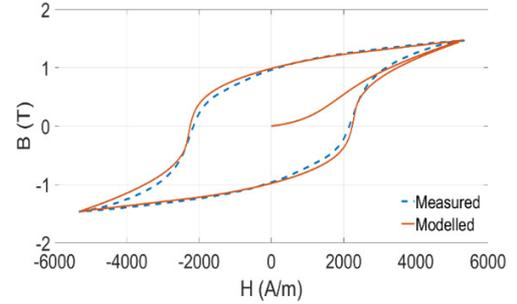
Fig. 3. Comparison of measured and modeled hysteresis curves at 1 mm Displacement for strip 3.
