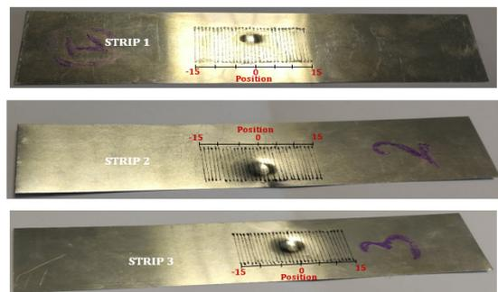
Fig. 1. Wrought iron strips subjected to surface treatment by hammering.
