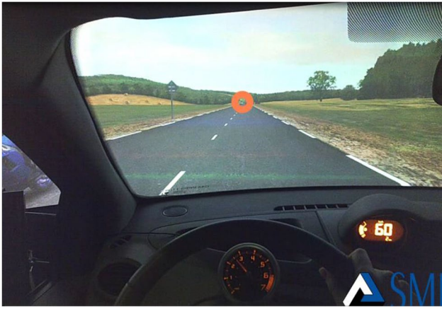
FIGURE 5 Calibration pattern for eye tracking.
