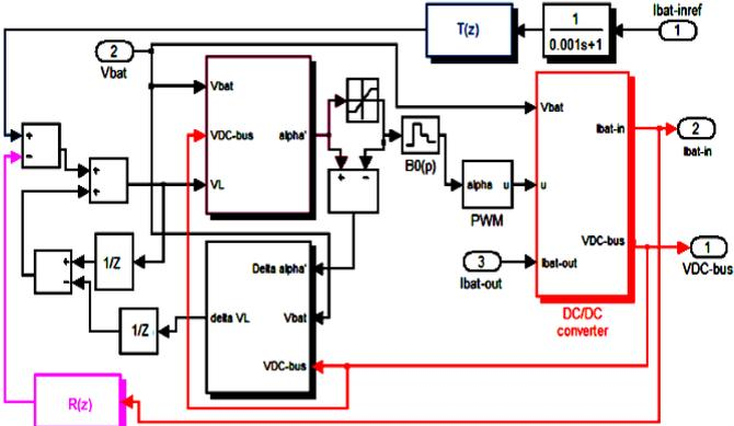
Figure.4.b: Battery's current control loop (inner loop)
