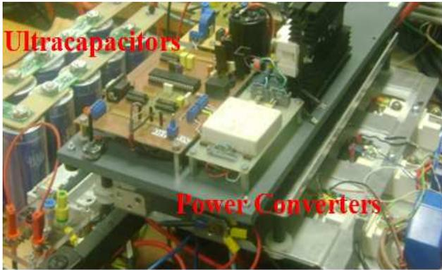
Fig. 14: Experimental setup for UC-lithium battery energy management.
