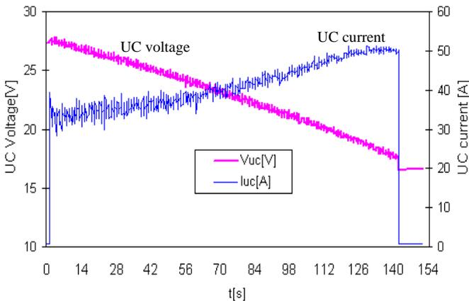
Figure 16: Ultracapacitors module voltage ( $V_{uc}$ ) and current ( $I_{uc}$ )
