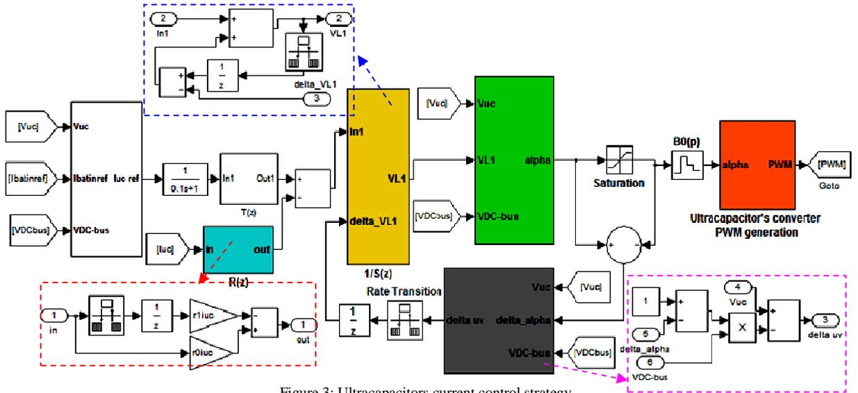
Figure.3: Ultracapacitors current control strategy
